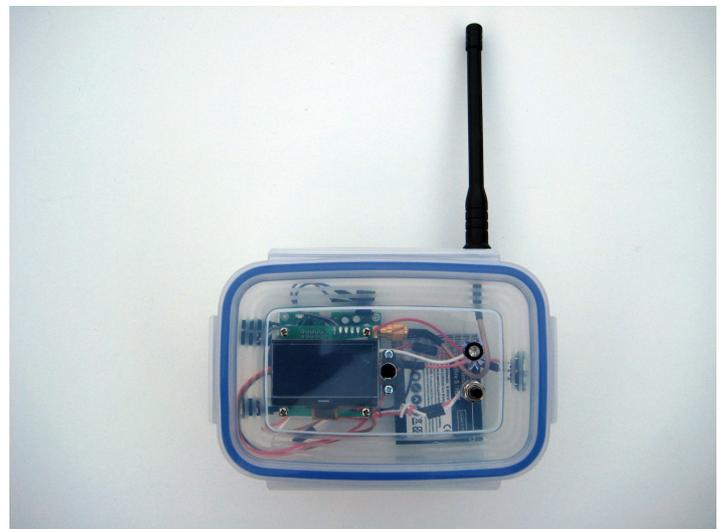
I have found the best displays for this type of application to be the small Digole serial 128×64 graphic LCDs. These are low power and some versions will run from supplies that can vary from 3v3 to 5V with no contrast adjustment needed as the supply voltage changes. These serial LCDs require only a single output pin from a micro controller to drive them. The 128×64 displays will show 7 lines of 21 characters at font size 10, there are other font options and graphics too.
