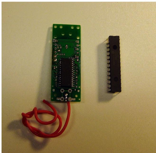
HABAXE2 used a PICAXE 28X2 and the Hope RFM98 radio transceiver. This Pico balloon tracker weighed around 16g with a 10g 380mahr Lithium Polymer battery and was attached to the 36" foil party balloon, filled with helium and adjusted for 2g of free lift, see picture below.
