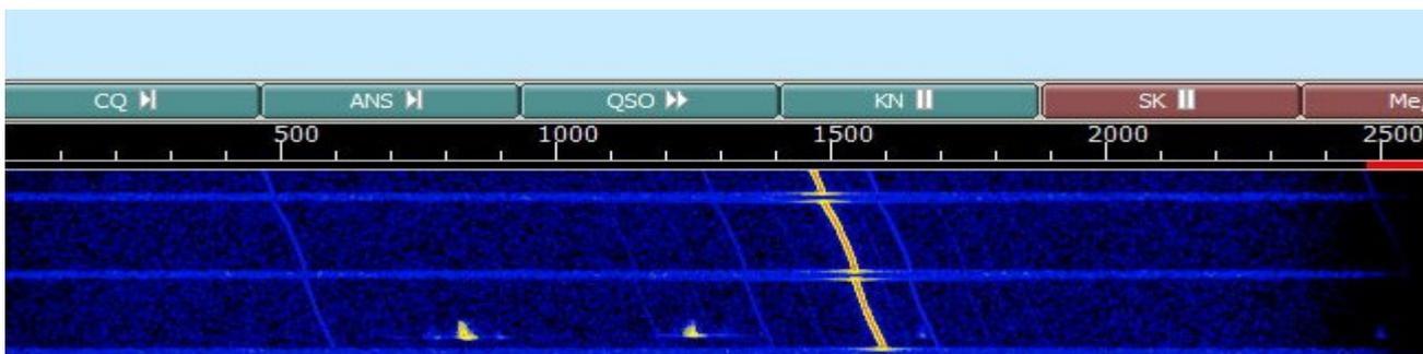
The problem (packets received with CRC errors) did not seem to occur with high data rate (1042bps) packets, but was present on the lower data rate (98bps) packets. It was also noted that the errors did not occur in short packets of 10 bytes or so, but did with longer ones. The problem also seemed worse with lower bandwidth packets.
