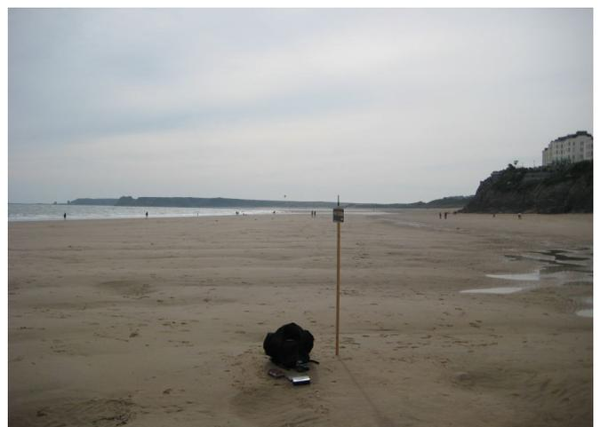
The testing principle here is simple, walk away from the transmitter until the beeps stop. The distance difference can then be converted into a dB performance ratio.
